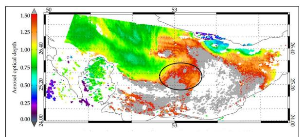
**Figure 2.** Aerosol optical depth (AOD) at 1km resolution over the Persian Gulf on 16 Sep 2008 as observed by AATSR. The radius 50km circle is centred on a concurrent Aeronet observation, which is used to validate the product.
